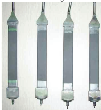
Fig. 1. Brazed anode-supported flat tubular cell with metallic cap by using BNi2 filler metal
