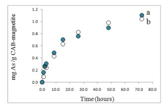
Figure 5: Sorption kinetics of Arsenate (a), and Arsenite (b), species on CAB-(DMSA)magnetite. The uptakes are expressed on a dry bead basis. The initial As concentration was 10.0 ppm
