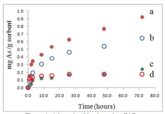
Figure 4: Adsorption kinetics using CAB-(DMSA)magnetite: Arsenate (a), Arsenite (b) and CAB: Arsenate (c), Arsenite (d). The uptakes are expressed on a dry bead basis. The initial As concentration was 5.0 ppm
