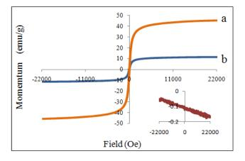
Figure 2: Room-temperature M-H loops for magnetite (a) and CAB-(DMSA)magnetite, 40% w/w (b). The inset corresponds to the M-H loop of bare CAB.
