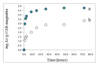
Figure 3: Adsorption kinetics of Arsenato (a), and Arsenite (b), species on DMSA-magnetite. The initial As concentration was 5.0 ppm.
