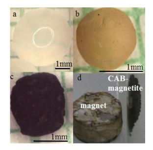
Figure 1: (a) 'Green'- CAB; (b) Dry CAB, (c) CAB-(DMSA)magnetite nanocomposite, and (d) CAB-magnetite nanocomposite in response to an external magnetic field.
