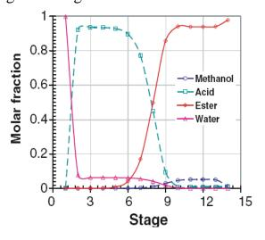
Fig.7.Reactive distillation column profiles- Liquid composition
