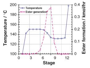
Fig.8 Reactive distillation column profiles- Temperature & ester generation
