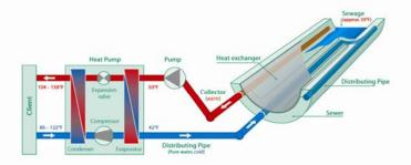
• Working principle of the Rabtherm waste heat utilization system
