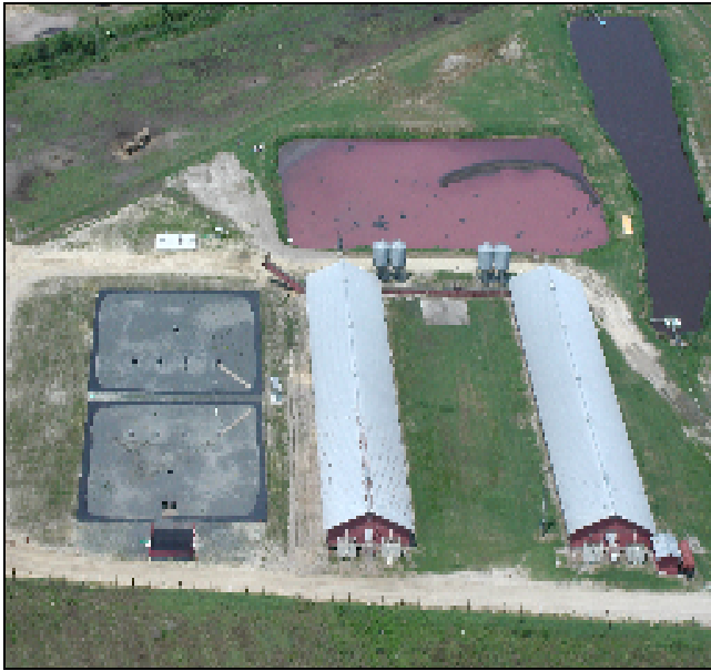
Figure 1. Aerial view of commercial-scale ReCip® demonstration for treating high strength wastewater from a confined swine operation. Based on independent studies performed by North Carolina State University: ( http://www.cals.ncsu.edu/waste_mgt/smithfield_projects/phaseIreport04/phaseIreport.htm ), this two-cell system was removing total nitrogen at an average rate approaching 200 pounds per acre per day.
