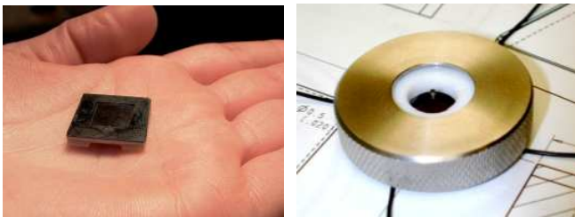
Figure 1. Example of the AlwaysReady Reserve Microbattery.as-made (left) and packaged (right).
