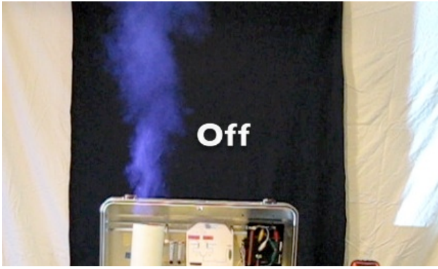
Test system burning rubber, showing particulate emissions. PAC disengaged .
