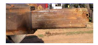
Figure 2: Continuous extrusion of compressed earth from small proof-of-concept machine.
