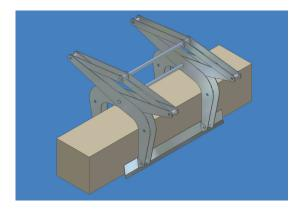
Figure 3: Isometric view of CEB lifter.
