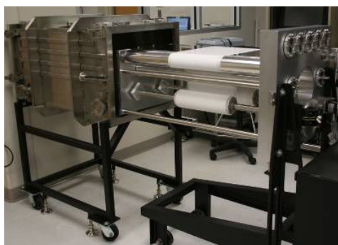
Figure 6. GVD has several on-site polymer deposition chambers suitable for coating a range of parts, including a roll-to-roll deposition chamber (shown here). coating technology is advantageous from both device fabrication and environmental standpoints.
