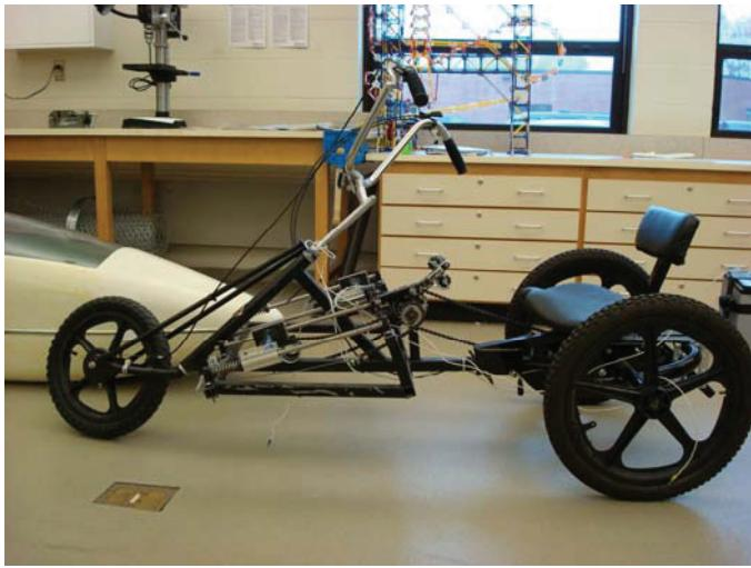
**Figure 1: Assembly of the trike without the top canopy holding the solar panels.**
