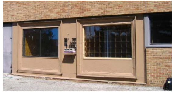
Figure 6. Full scale thermal chambers showing the typical double glazed low e coating window on the left and the SITumbra composite panel on the right.
