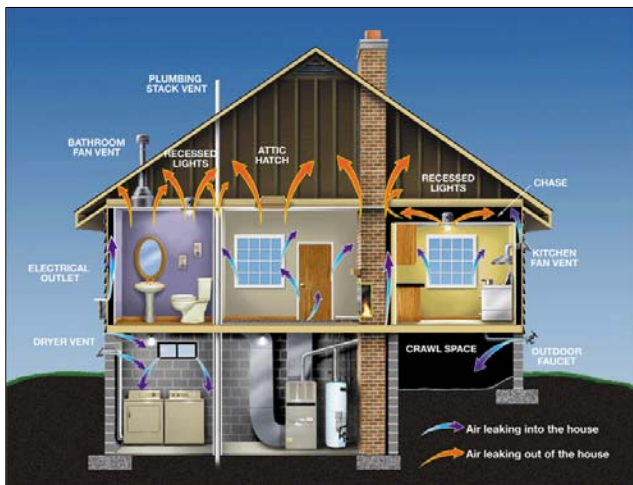
Fig. 1 Common Sources of Air Infiltration Source: U.S. Environmental Protection Agency
