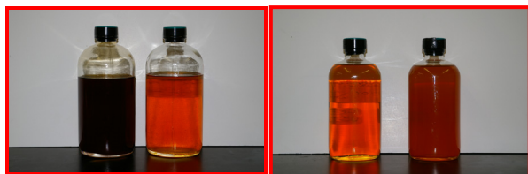
Figure 5: (a) Image of thermally degraded biodiesel fuel before and after removal of FDP using Seldon's Nanomesh™ filter; (b) Image comparing the effect of a traditional filter against the effect of Seldon's Nanomesh™ filter for the removal of FDP from commercial diesel fuel.
