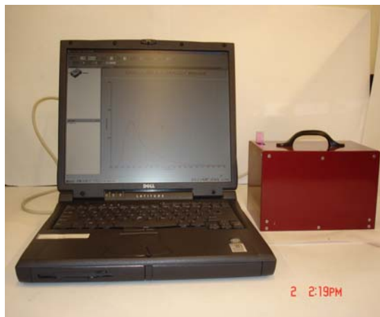
Figure 4: Photograph of the minimized NSET probe box, connected with laptop computer for data acquisition.
