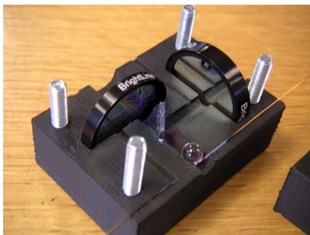
Figure 2. The epifluorescent detector – note the capillary running along the front edge of the device beside the sapphire ball lens.
