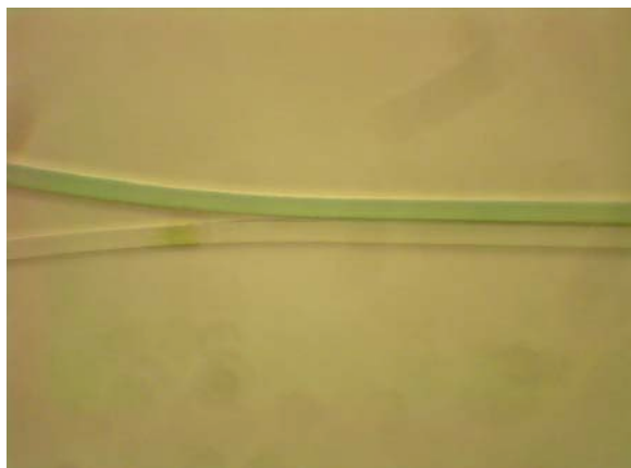
Figure 3. Laminar flow of two phase systems containing diesel and an aqueous extractant
