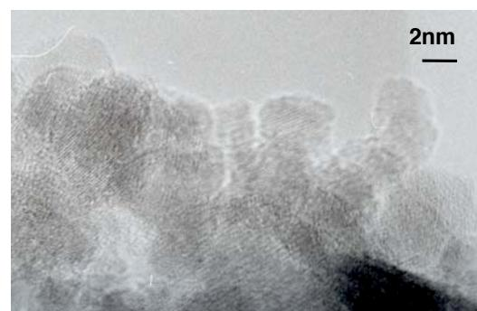
Figure 2: HRTEM image of the highly crystalline structure magnetite/maghemite in silica.
