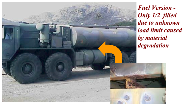
Figure 3. Fuel version of HEMTT with corroded supports
