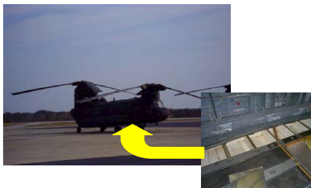
Figure 2: CH-47 Chinook Corrosion Under Floor Boards
